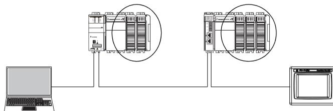
Remote I/O modules accessible by using a 1769-AENTR EtherNet/IP adapter
