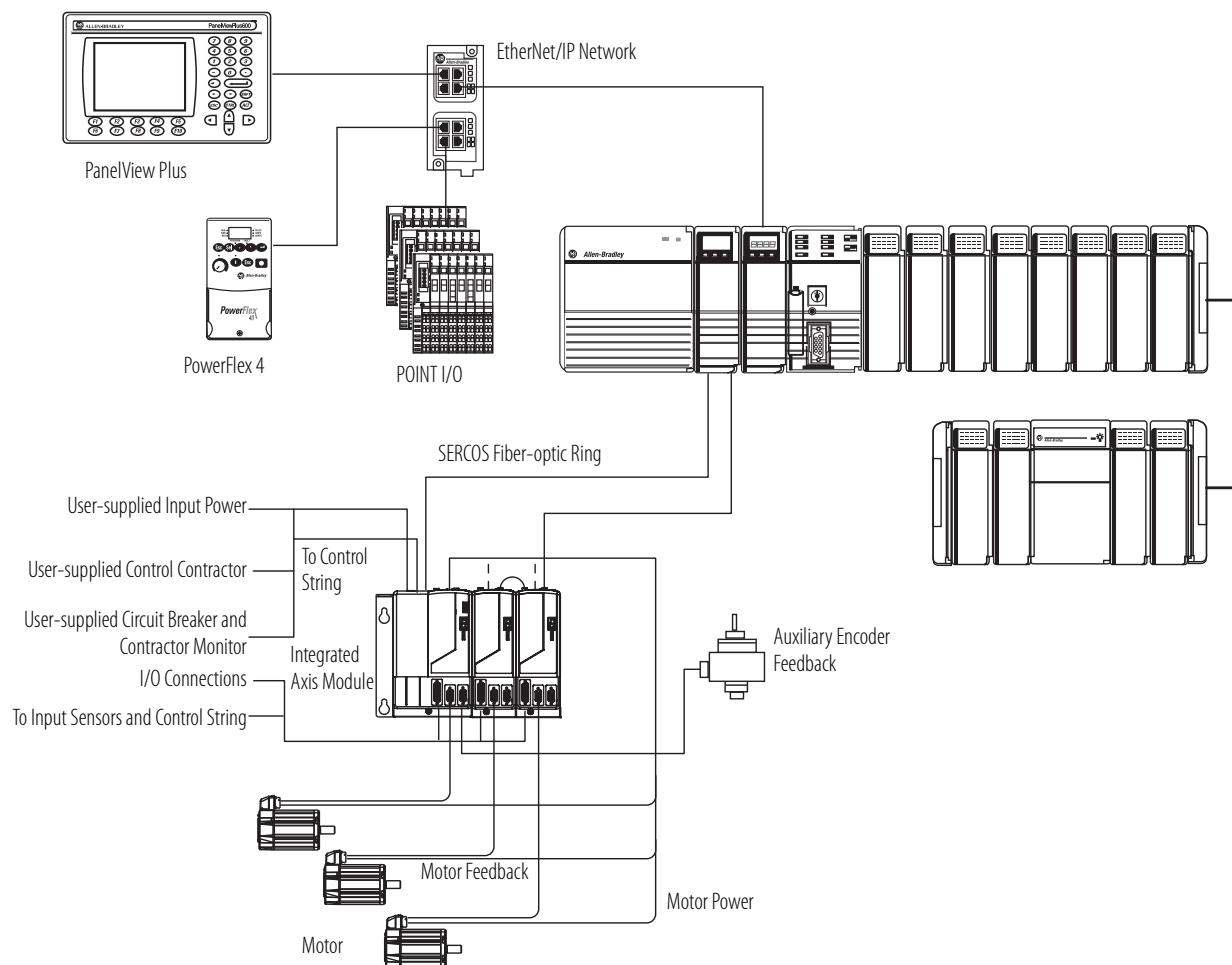
**1768 CompactLogix Controller and Four-axis Integrated Motion with Kinetix Drives and LIM Interface**
